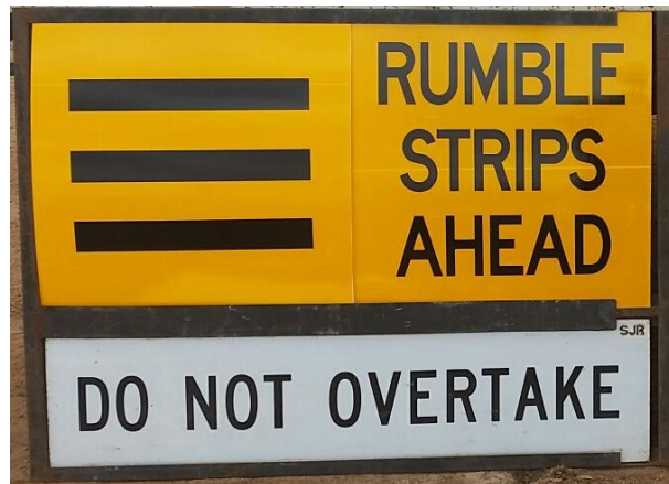
Fig 3. Multi message sign configuration
