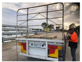
9.2 Once the rear gate has been removed, secure it to the front gate on the vehicle via ropes.
